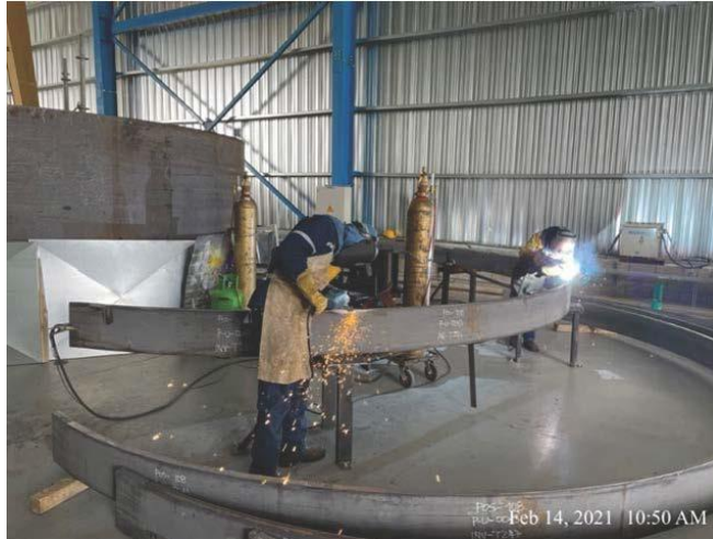
Figure 56: Lower elbow: steel lining element manufacturing
