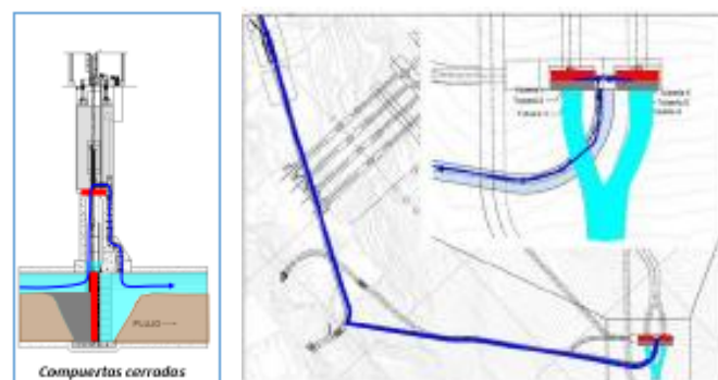
Figure 60: GAD gates in their final position with temporary direct by-pass system (left) and through the IDG (right)
