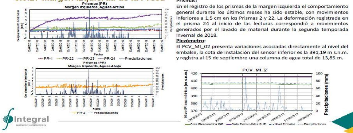
Figure 31 – Left abutment. Geodetic monitoring since June 2018 stability. No signs of deformation to be considered, no trend.
