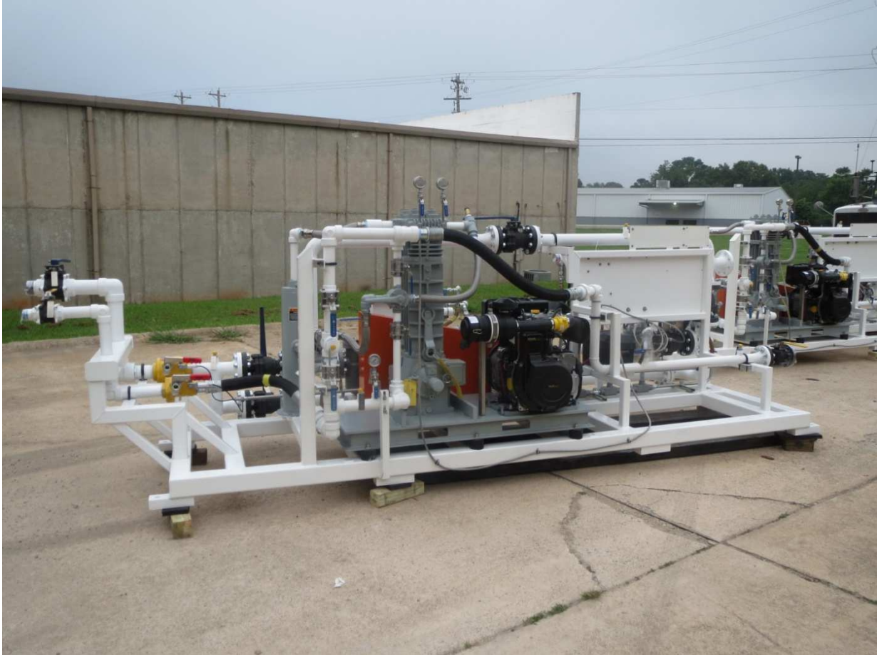
Photograph #18: Example of Skid Mounted LPG Loading Facility.
