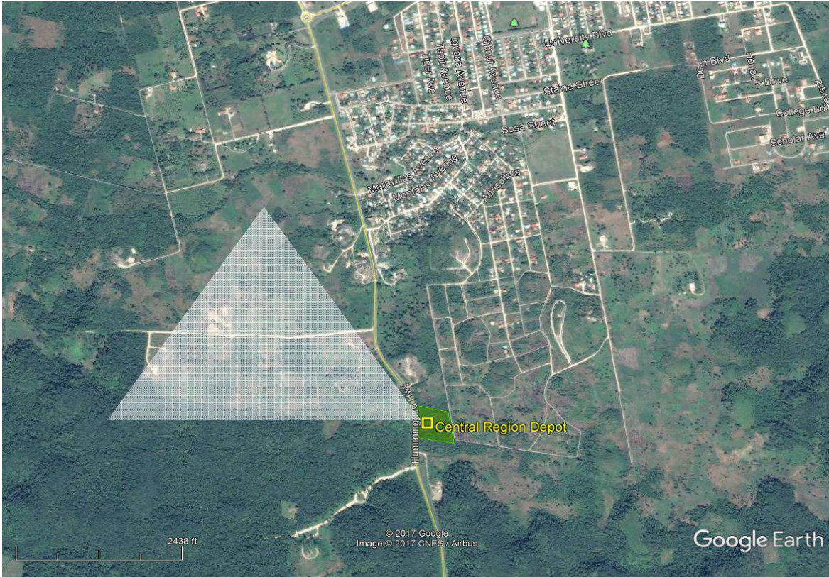
Figure 37A: Area predominant winds would carry released LPG - Central Region Depot.
