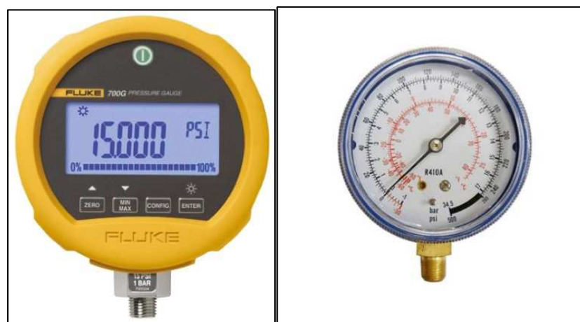
Figure 26 & 27: Examples of Different Types of Digital and Analogue Gauges
