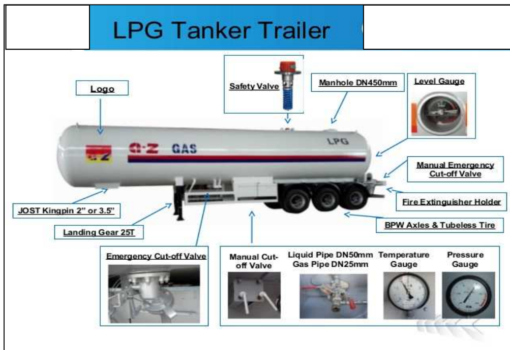
Figure 64: LPG Tanker Trailer with Safety Devices
