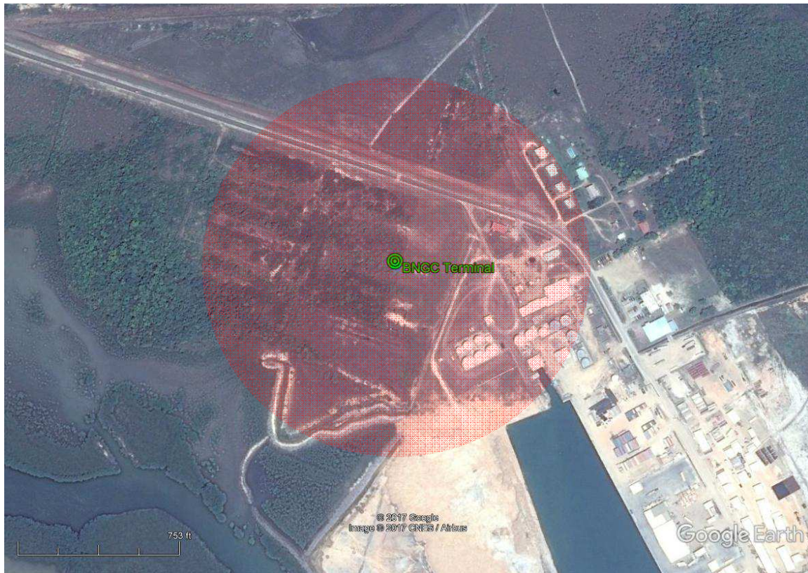
Figure #42: Estimated 300 meter Zone of Influence with greatest impacts in a BLEVE incident.
