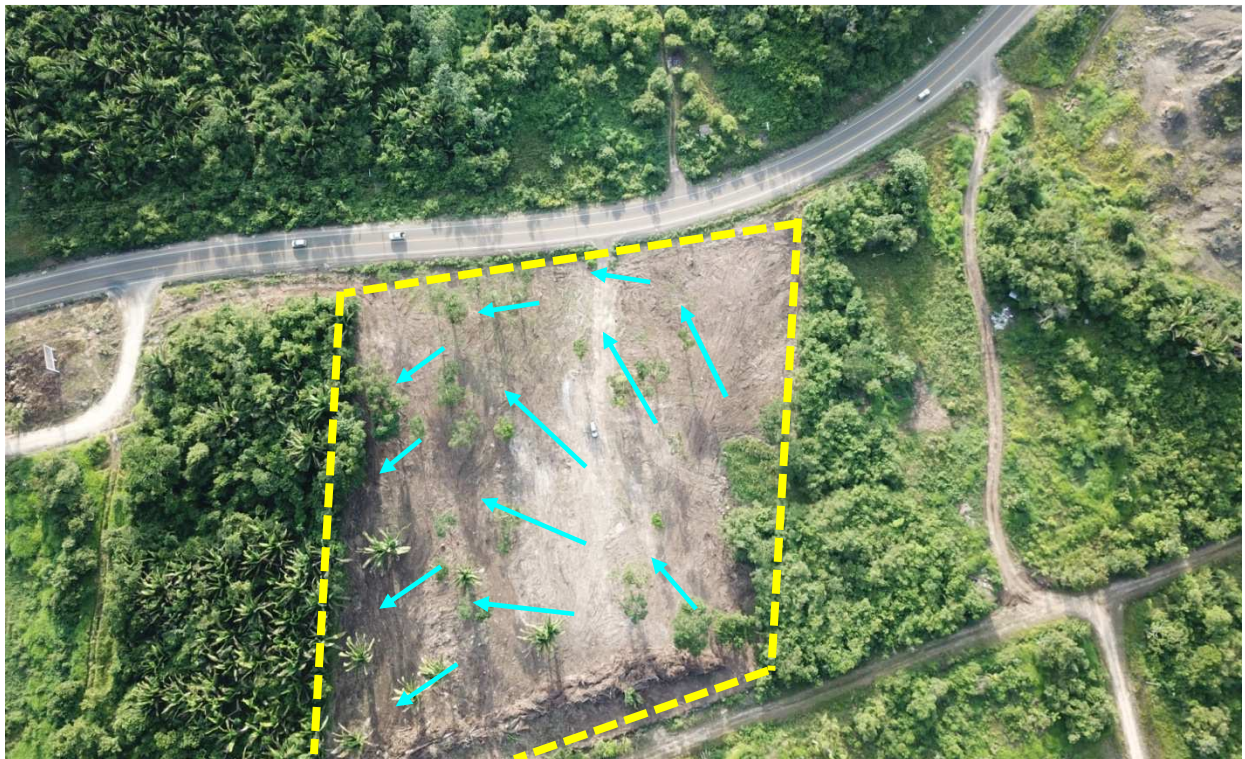
Photograph 36A - Flow of drainage at Central Region Depot Site (top of picture is west)
