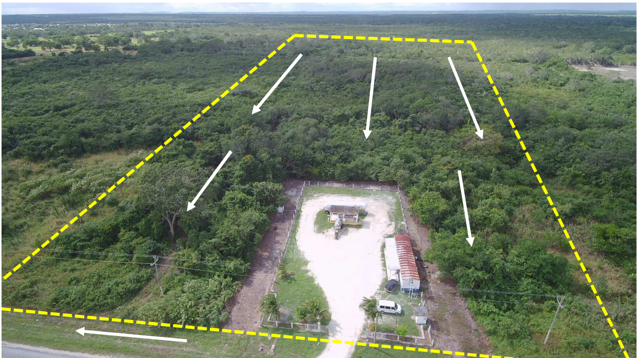
Photograph 36C - Flow of drainage at Northern Region Depot Site (top of picture is west)
