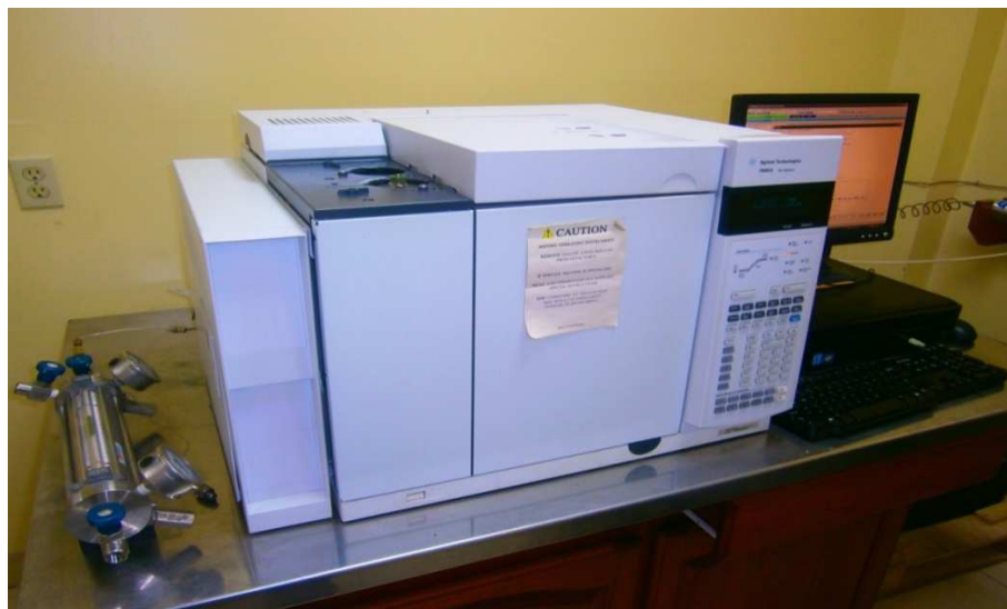
Photograph 14 – Gas Chromatographer used in Laboratory Analysis of LPG Blends
