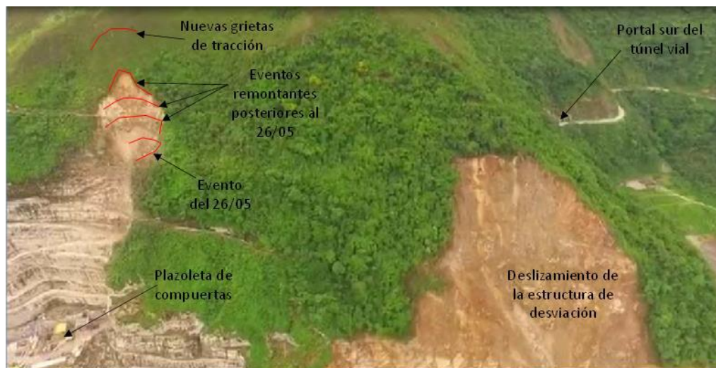
Figure No.12: "El Romerito" landslide. Photo 28/05/2018 (from ppt Prof. G. Fernandez, June 2018)
