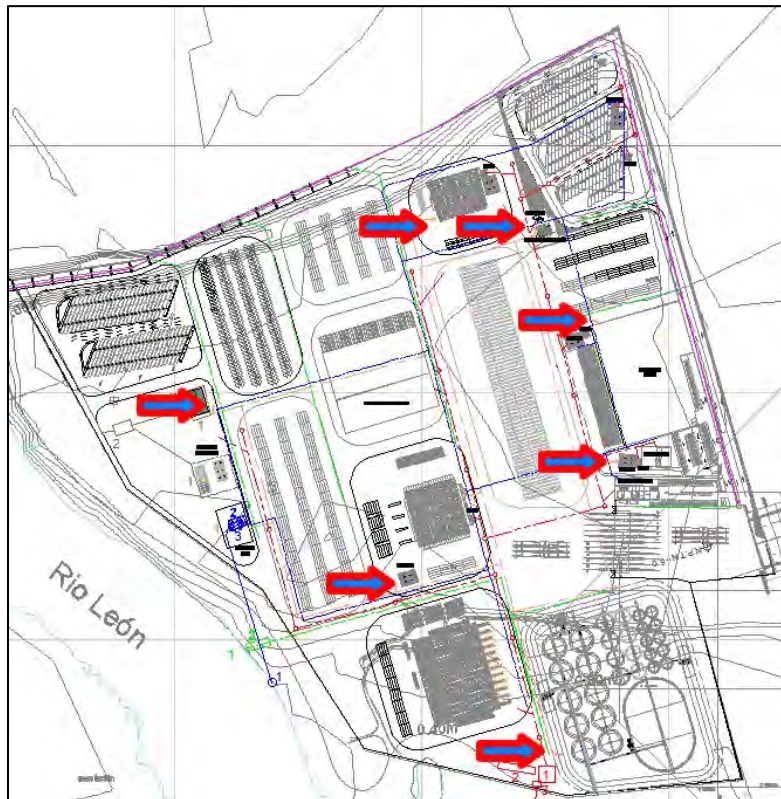
Figure Num. 3.33. Location of valves for sectorization of the fire network, red arrow with blue
